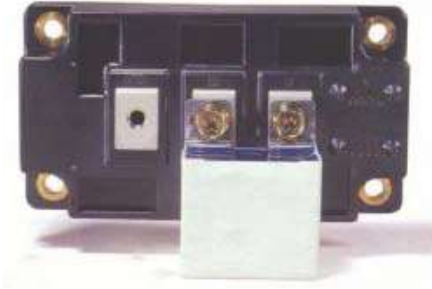
Fig. 2 IGBT with MDirect Mount™ Snubber Capacitors
